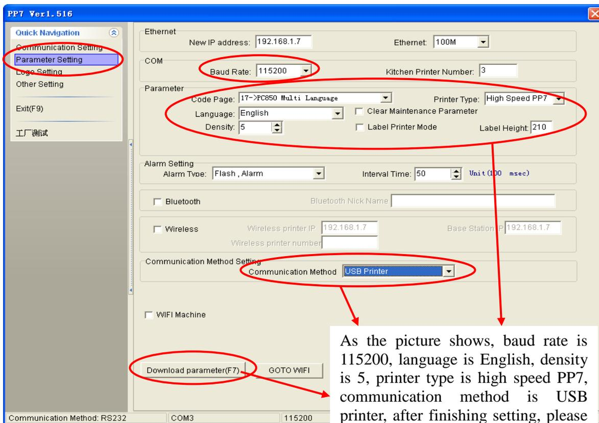
As the picture shows, baud rate is 115200, language is English, density is 5, printer type is high speed PP7, communication method is USB printer, after finishing setting, please click download parameter.
